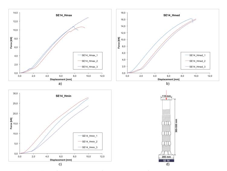
Figure 1 Diagram force versus displacement of testing machine's crossbar for Hmax (a), Hmed (b), Hmin (c) and typical "Eterno SE14" specimen (d).
