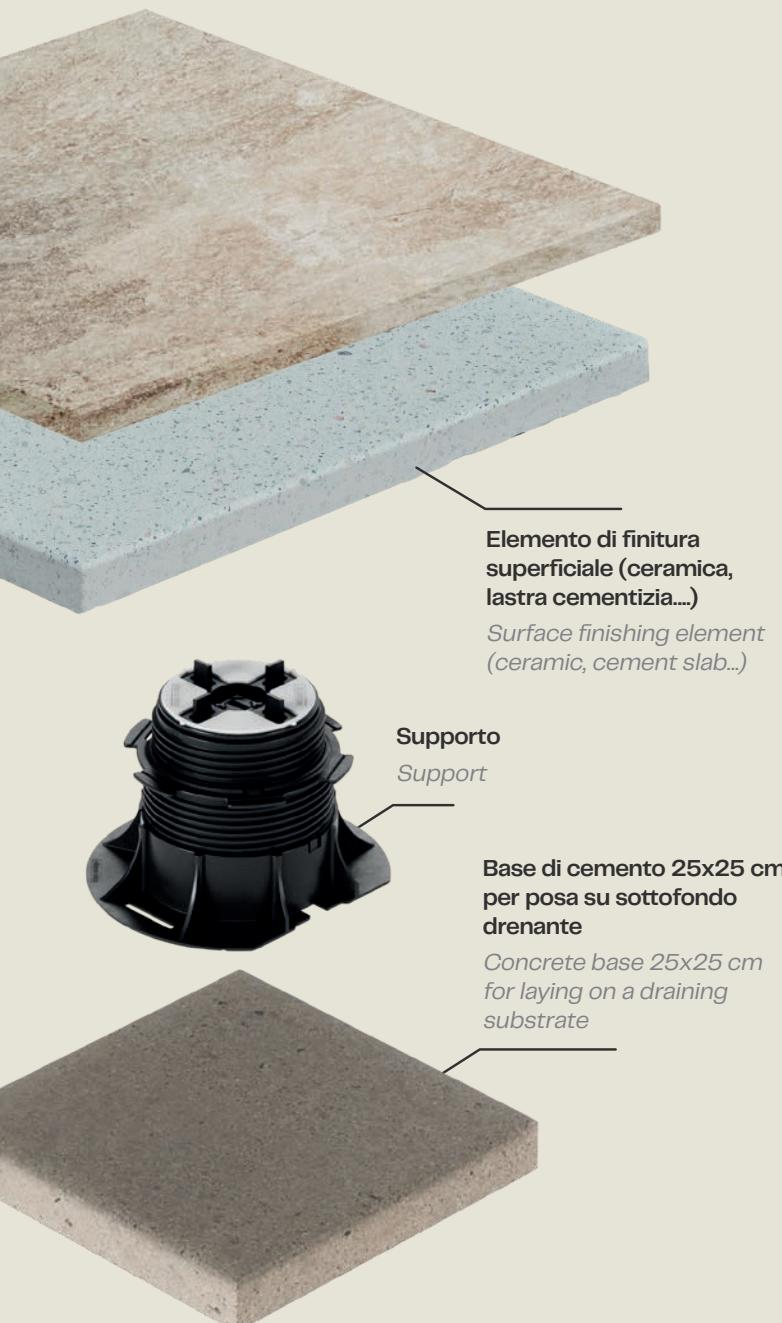
Floors raised with the Pedestal system are made using ceramic, concrete, or natural stone slabs. Unlike decking, to install these floors, you only need to use fixed or adjustable supports to compensate for height differences from the base to the elevated floor level. The slabs are placed directly on the supports, and the floor is ready to be used – no additional support structure is required.
